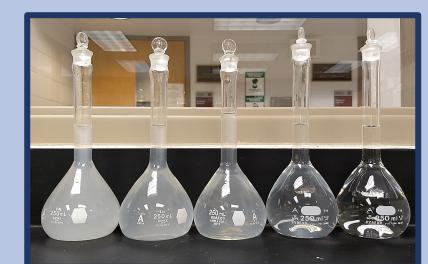
Initial data supports device function over a range of turbidities typical of small streams. Preliminary results indicate a linear detector response with R<sup>2</sup> = 0.96. More data is necessary to statistically validate results.
