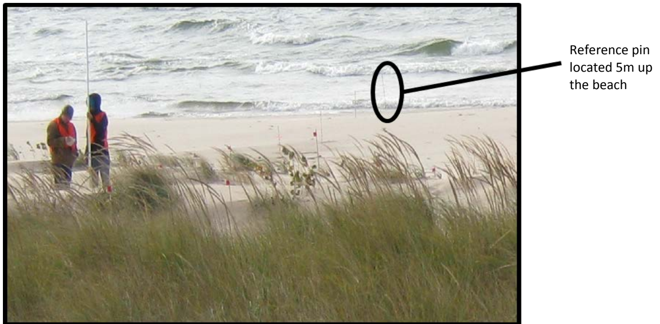
Figure 15: Wave run-up reaching the 4 th pin in a line of 5; pins are spaced 5 meters apart.
