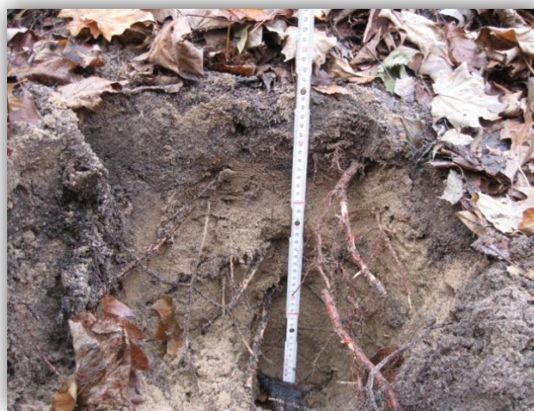
Figure 11: This soil pit on the leeward slope of the dune displays distinct soil horizons.
