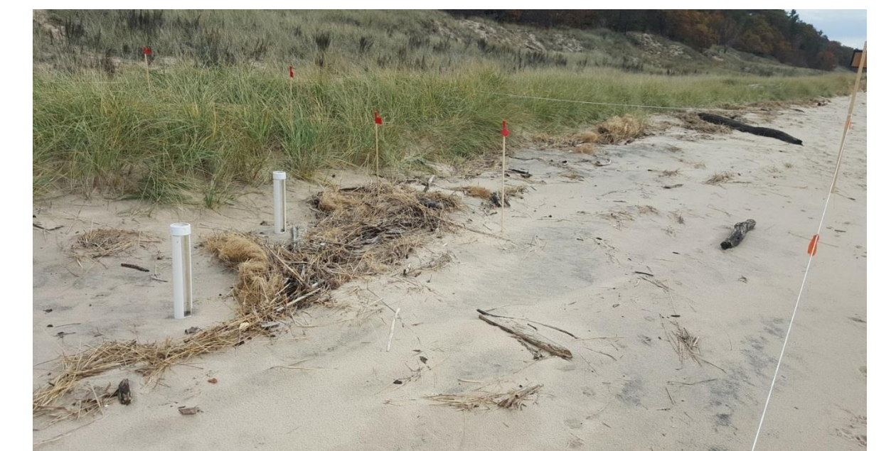
Figure 5. Wrack on portion of the study area at Hoffmaster State Park. Note the erosion pin and sand trap placement.
