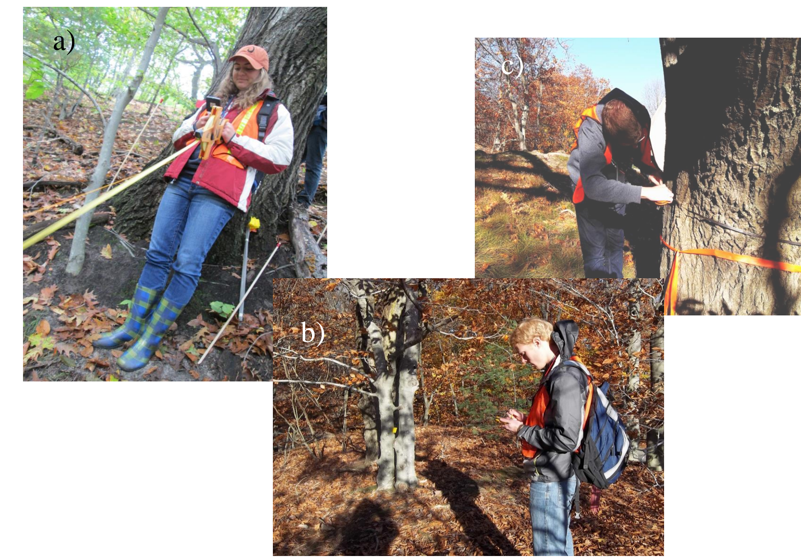
Figure 2: Researchers a) measuring the study area's 50m radius, b) recording tree data using GPS, c) measuring the diameter at breast height of infected oaks.
