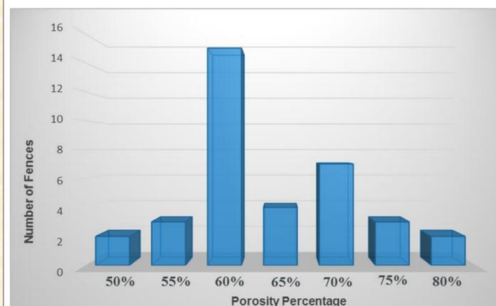
Figure 4: Porosity of studied sand fences. No fences observed at the study sites had porosities of less than 50%.
