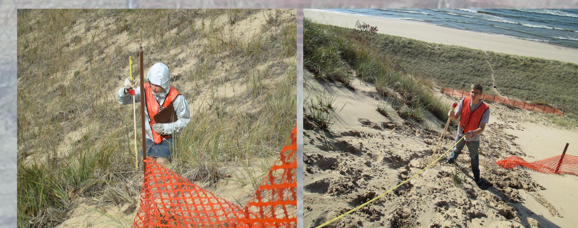
Fig. 5A Measuring Erosion Pins
