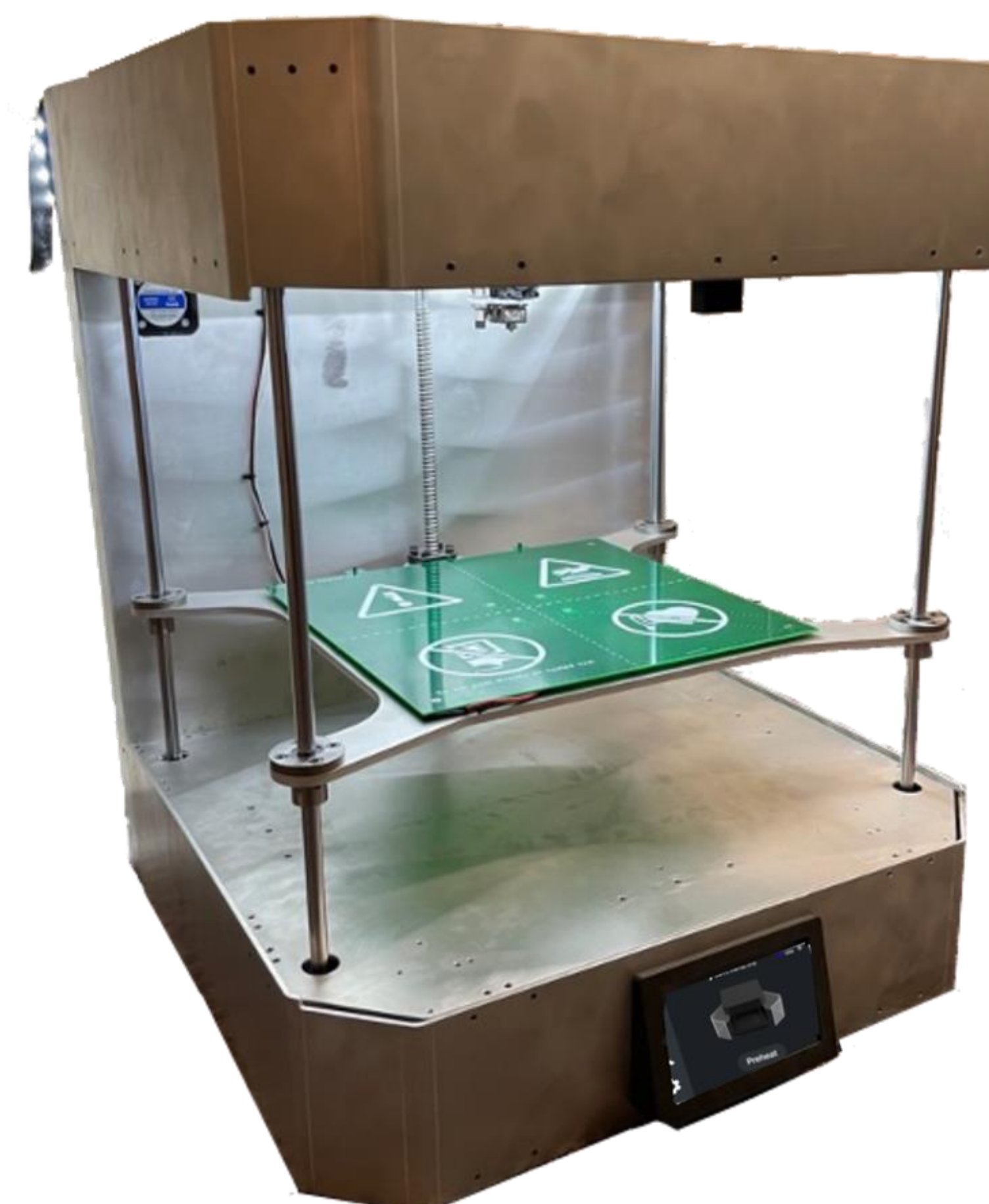
The printer, before walls and door are placed.
